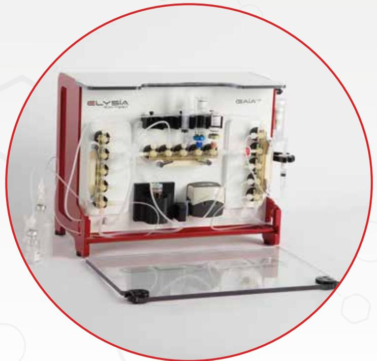
Gaia V2 is the second generation of our synthesis unit for the labeling of peptides such as DOTA-TOC or PSMA with radioactive metals (e.g.  $^{68}\text{Ga}$ ). The design was reworked to reduce the size to a maximum and optimized to provide a fast, simple and intuitive production of common radio tracers. The position of the connections has been modified to reduce the need for space in the Hot Cell and to improve the accessibility for maintenance.
