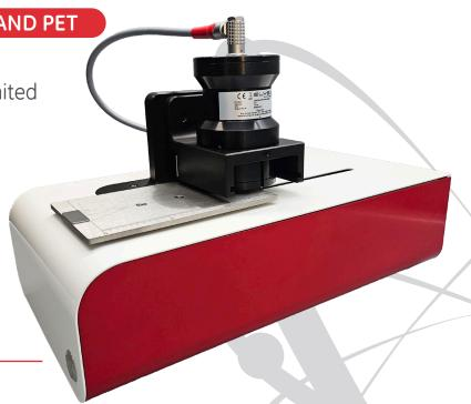
The miniGITA Slim is the new version of the well known miniGITA Single. Its size has been reduced to fit the actual space constraints of modern laboratories. Its small footprint allows it to be used in a laminar air flow or an isolator. This was achieved by optimizing the internal mechanics without compromising the measurement technology. The new Slim can use the same detectors and collimators as the miniGITA Single or Dual and achieves the same excellent measurement performance.
