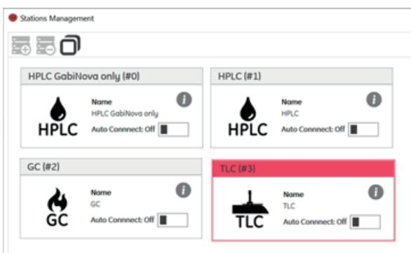
GINA X is able to control several chromatography systems at the same time. With one PC or user access point you can control several HPLC's or other chromatography systems such as a GC or our miniGITA. The user-friendly interface allows a simple overview of all available systems and makes the lab management easier.
