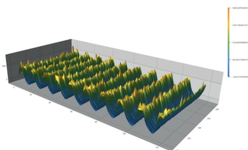
This module is needed for the data acquisition from a Diode Array detector. It allows to show the complete data set from the DAD measurement in a 3D Graph. Simply track your mouse over the 3 D Spectrum to find the regions of interest. The software will show you in a 2D window the corresponding spectrum and chromatograph.
