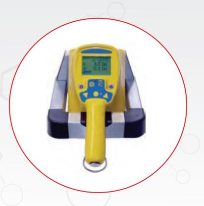
CoMo 170 is a portable contamination monitor for  $\alpha$ ,  $\beta$  and  $\gamma$  surface contamination. The detected events are counted over time and displayed digitally in c/s, Bq or Bq/cm². Measurement results can be stored and transferred by RS 232 C.
